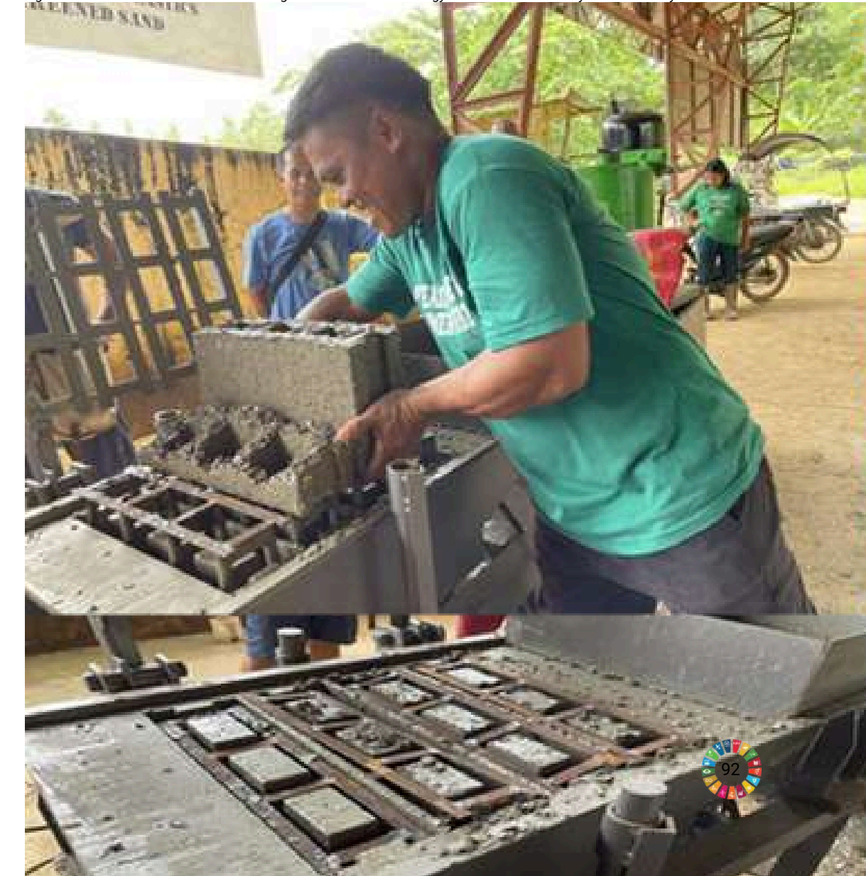
Figure 79. Fabrication of Hollow Blocks using the Alternative Technology installed in the Sanitary Landfill Facility
